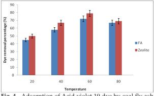
**Fig. 4.** Adsorption of Acid violet 19 dye by coal fly ash and zeolite at different temperature.
