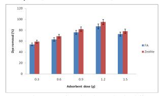
**Fig. 2.** Adsorption of Acid violet 19 dye by different adsorbent dose.
