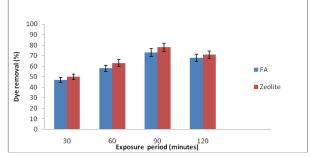
**Fig. 1.** Adsorption of Acid violet 19 dye by coal fly ash and zeolite at different exposure period.
